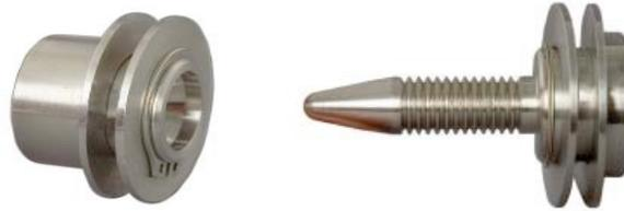
As you can see in the photo below, the female-segmented threads are held together by the garter spring. The garter spring keeps the concentric threaded female segments around the male component. Once inserted, any force pulling the male component will cause the female to clamp tighter due to the chamfered angle cut in the leading end of the male threaded segments and the corresponding cut in the Zip-Nut body.
