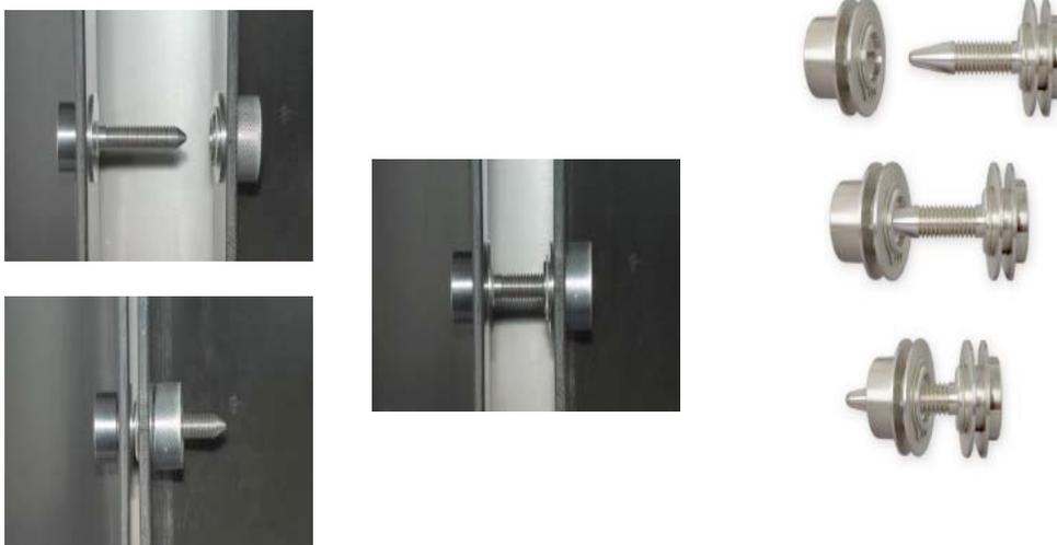
The photos below illustrate the special thread design of the fastener components. To prevent loosening due to vibration or rotation, radial grooves cut in the male components replace the helical threads normally used in fasteners.
