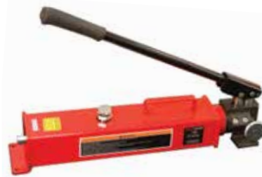
150H 10,000 psi. 2-stage manual hydraulic power unit delivers 0.66 in 3 /min. @ 325 psi. and 0.16 in 3 /min. @ 10,000 psi.
