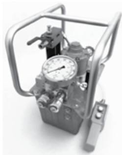
FHFA-10K 10,000 psi. compact air driven hydraulic power unit delivers 620 in 3 /min. @ 0 psi. and 62 in 3 /min. @ 10,000 psi.
