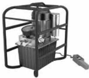
FHFE-10K 10,000 psi. compact electric driven hydraulic power unit delivers 620 in 3 /min. @ 0 psi. and 62 in 3 /min. @ 10,000 psi.
