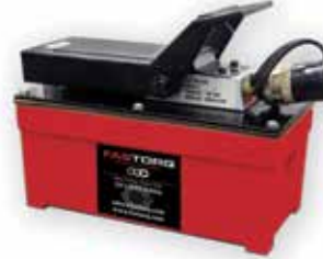
105A 10,000 psi. air driven, foot actuated hydraulic power unit delivers 68 in 3 /min. @ 0 psi. and 4 in 3 /min. @ 10,000 psi.
