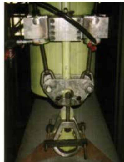
Figure 4. An example of In-Situ Hanger Test Assembly.
