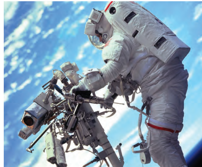
Astronaut Steven L. Smith, payload commander on STS-103, stands on the mobile foot restraint at the end of the remote manipulator system (RMS). ZipNuts were used to service the Hubble Space Telescope during this December 1999 mission. Image credit: NASA
