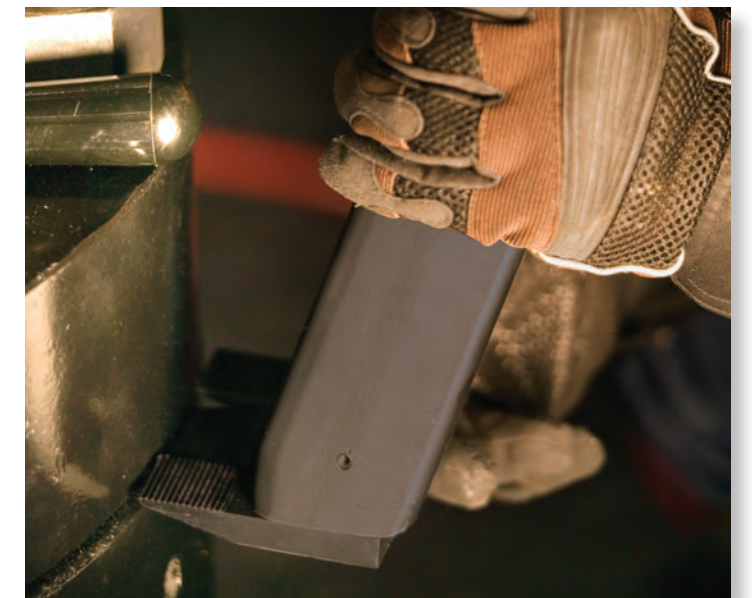
The serrated feet on AutoSPREADER keeps it in place and only needs 3/16" of space to insert.
